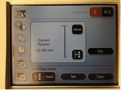
The z control moves the objective nosepiece down (closer to the sample) and up. Home is set to the top position, holding the home button will move the objective up.
